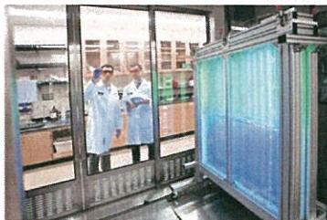
Process-scale photoredox flow reactor at Merck
